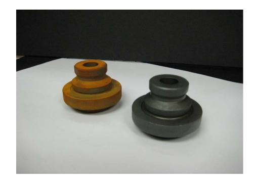
**Step 7:** 3:30 p.m. Cleaned part (at right) is dry and corrosion-free.
